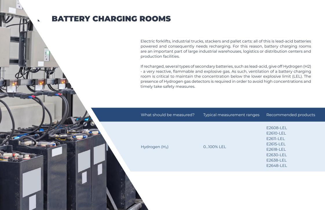
The correct operation and increase in life-time of the secondary batteries also require proper temperature and humidity, which can be achieved by using special measurement instruments.
