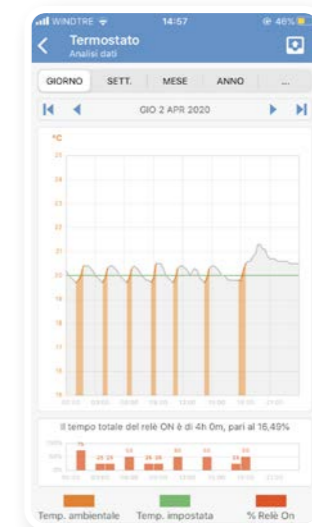
Control of heating system: on/off status, set temperature and measured temperature.
