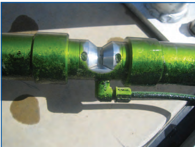
spectro::lyser with efficient automatic air cleaning
