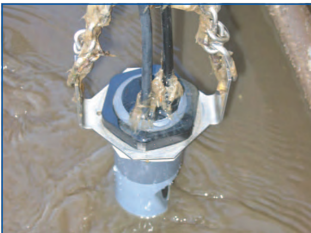
oxi::lyser in aeration tank
