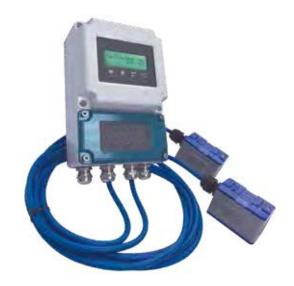
These flowmeters operate on the ultrasonic pulses transit time difference principle. The great advantage is the mechanical installation, because it is not necessary to cut the pipe. The sensors are simply clamped on the outer pipe surface, for this reason the pressure and the liquid aggressiveness to be measured are not a problem for the fl owmeter. The system measures in a bidirectional way and is suitable for clean or slightly dirty liquids.
