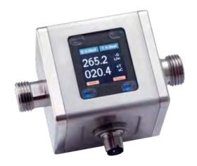
Measuring device suitable for measuring values from a minimum of 0.04l / m (DN5) up to a maximum of 100l / m (DN15). The body totally in AISI 316L makes or instrument suitable also for chemical / food applications. The reduced dimensions and the variety of threaded connections allow an easy and quick mechanical installation. Rotating the display of the TFT display allows horizontal or vertical mounting orientation.
