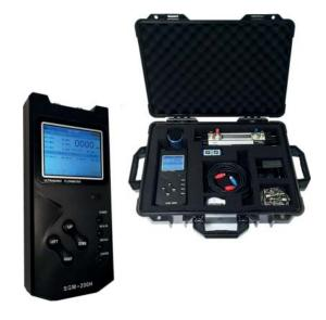
The flowmeters operate on the ultrasonic pulses transit time difference principle. The great advantage is the mechanical installation, because it is not necessary to cut the pipe. The sensors are simply clamped on the outer pipe surface, for this reason the pressure and the liquid aggressiveness to be measured are not a problem for the flowmeter. The system measures in a bidirectional way and is suitable for clean or slightly dirty liquids
