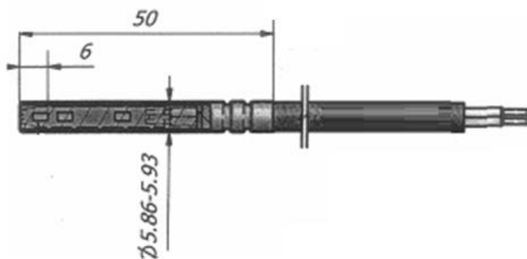
Fig. B3.2 Overall dimensions of the PL type temperature sensor
