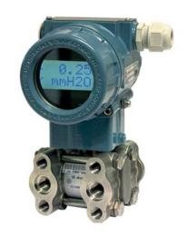
It is a differential pressure transmitter with performance at the top of the range and is designed for specificinstallations in processes where accuracy and stability over time are essential characteristics. Thanks to its technology it measures very low differential pressures from 1 mbar (10 mm H2O). It is fully programmable by means of two external watertight buttons and a matrix backlight display.
