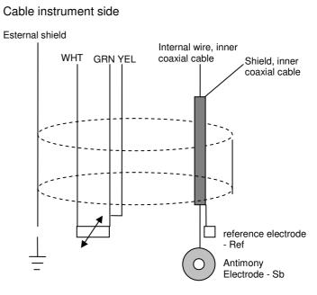
Wiring inside the probe
