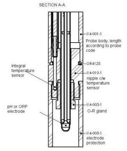
The calibration can be operated either by comparison to properly calibrated portable instruments or extracting the probe from the process liquid, cleaning it and then immersing it into the solutions with known value of the parameter to be calibrated. Calibration frequency is to be defined by the operator according to specific process requirements.
