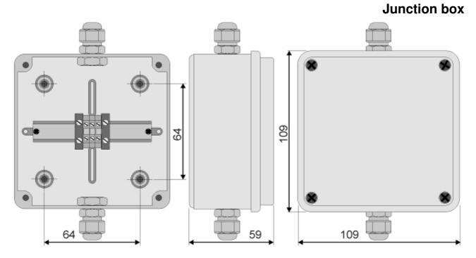
Junction box for the connection of one or two sensor to a remote transmitter. The number of terminals depends upon type and number of sensors to be connected. Cable glands for cable inlet and for cable outlet assure IP65 protection degree.
