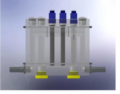
thermo compensation and the system for automatic sample flow rate adjustment. The electrodes are directly immersed into the sample that flows in the chamber with a constant flow rate, controlled by the cell itself; the electrodes are kept clean and active by the movement of the sample itself.
