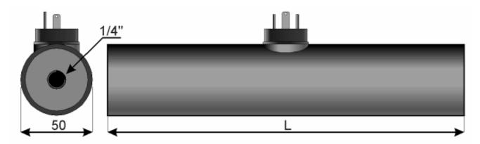
Conductivity cell with hollow cylindric PVDF body, graphite electrodes. Cell constants are K = 0.1 cm and K = 0.01 cm, and measuring ranges are  $0 \div 200$  mS and  $0 \div 2000$  mS. All 401C cells include integral temperature sensor Pt100, Pt1000, TC100 or other upon request, for measure thermo compensation. Process connections are  $\frac{1}{4}$  F suitable for direct installation in closed pipelines.
