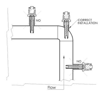
Series 401J cells should be installed at the minimum immersion depth indicated in figure, and the immersion depth should be kept reasonably constant. In process applications the sample flow should be directed against the cell bottom so that the liquid entering the cell can flow upwards
