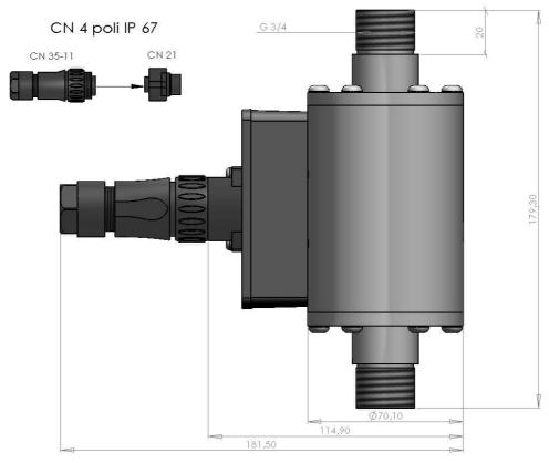
Hollow conductivity cell, cylindric body, AISI 316 stainless steel, with graphite electrodes. Cell constant is K = 1 cm, and measuring range is  $0 \div 100000 \,\mu\text{S}$ .
