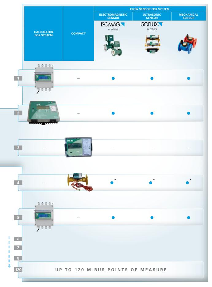
Any meter for any kind of measurement (e.g. gas, electricity etc..) if provided by Mbus protocol can be connected to the DMT.
