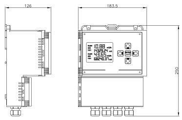
Level, open channels flow and pumps control unit
