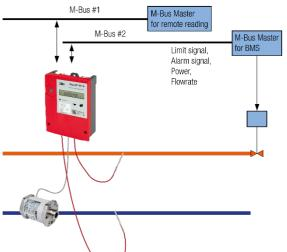
The M-Bus has established itself as the standard for meter reading as it has been standardised in EN 13757, and offers a variety of other features.
