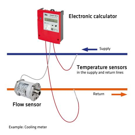
The thermal output (P) of a pipe-conduit network is based on a measurement of the flow temperature, return-flow temperature and volume flow of the heat transfer medium.
