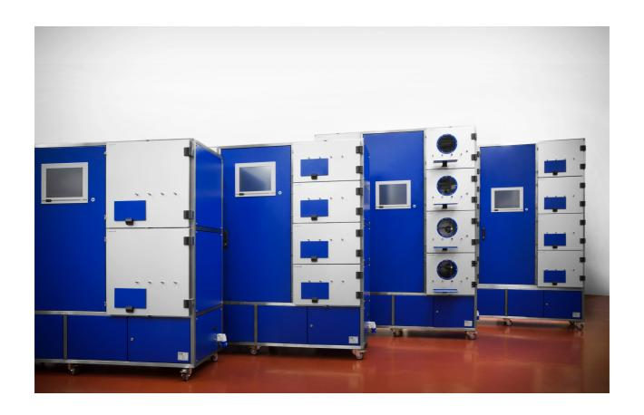
VOC Emission Test Chambers according to EN ISO 16000-9, UNI CEN/TS 16516, GEV Testing Methods, UNI EN 717-1, ASTM D5116
