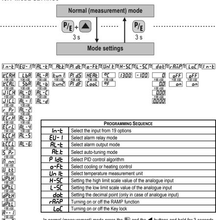
In normal (measurement) mode press the **№** and the **d** buttons and hold for 3 seconds to change the mode settings. If the configuration is completed press the **№** button and hold for 3 seconds to return to normal (measurement) mode.
