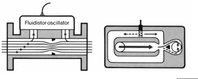
The right hand picture shows a cross section of the fluidistor. The gas flow enters the meter on the left and leaves it through the connection to the right.
