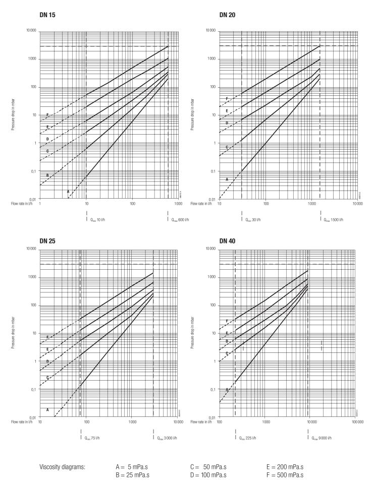
For a pressure drop of more than 1 bar, it is recommended to use the next larger meter size. Maximum permissible pressure drop = 3 bar
