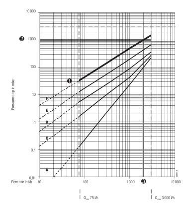
Mineral oil, viscosity 450 mPa.s VZO 25 mounted on pressure side of pumps
